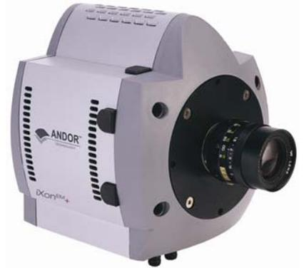
This new 1024x1024 frame transfer format offers unequalled thermoelectric cooling down to -95°C, industry-lowest clock induced charge noise, and operates at 9 frames/sec (full resolution). EMCCD and conventional CCD readout modes provide heightened application flexibility.
