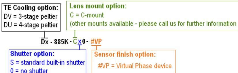
E.g. a DV-885K-C00-#VP is an iXon<sup>EM</sup> + 885 camera with 3-stage peltier vacuum cooling and without internal shutter.
