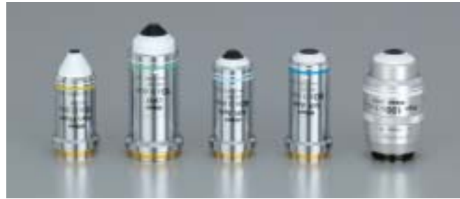
CFI Plan Fluor 10x W, NA 0.3, W.D. 3.5mm CFI75 LWD 16x W, NA 0.8, W.D. 3.0mm CFI Apo 40x W NIR, NA 0.8, W.D. 3.5mm CFI Apo 60x W NIR, NA 1.0, W.D. 2.8mm CFI Plan 100x W, NA 1.1, W.D. 2.5mm
